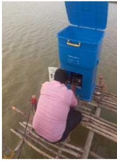
Automatic feeder is little bit weight and weighs about 15 kg and it makes very easy for fixing and control. Feeders motor consumes 50 watts only and its 10 -15 times lesser than the consistent auto feeder and it can consume around 220 - 240 watts. It can disperse at the maximum rate of 1.2 kilograms per minute and up to 2,000 times per day or every 45 seconds.
